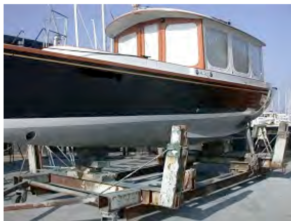
Nontoxic, ceramic-epoxy hull coating in very good condition after 13 months
