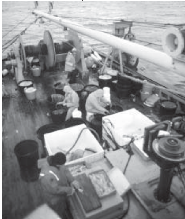
Sablefish longliners unfurl lines a mile in length with hooks every 15 to 20 feet. Photo: John Bortniak, NOAA Corps.
