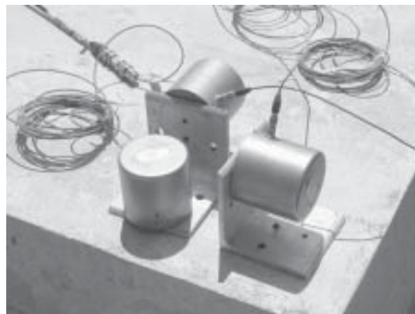
Instruments called accelerometers record how the pier moves in response to an applied force. By placing three of these instruments at right angles to each other, all accelerations in the horizontal and vertical directions are recorded.
