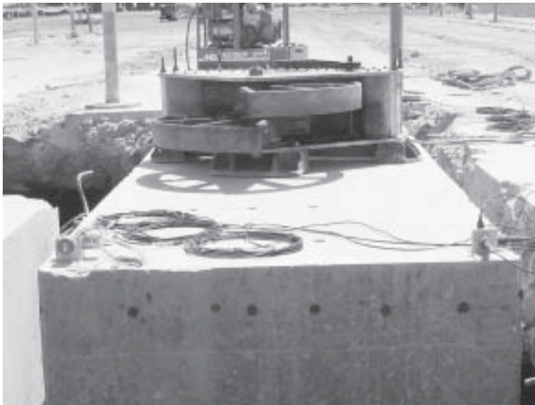
A 5,000-pound rotating shaker vibrates sections of the pier at different frequencies to identify the structure's natural harmonics from which structural characteristics such as stiffness are inferred. More vigorous shaking simulates ground motions that might be felt during an earthquake.
