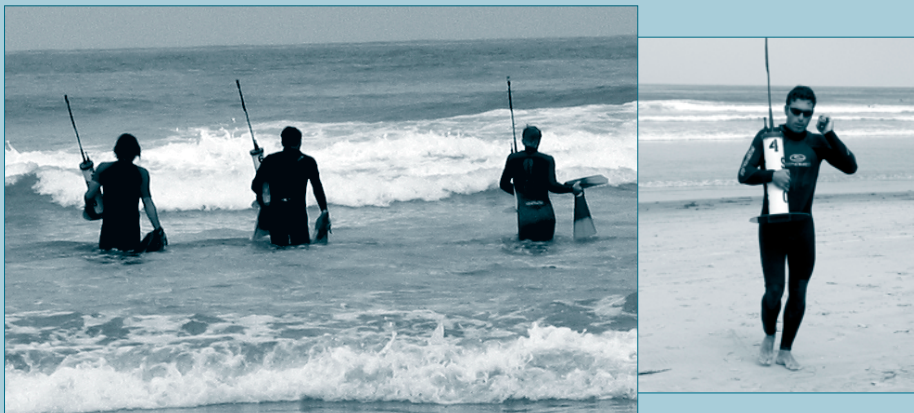
With Sea Grant funding, oceanographers have built the first ever satellite-tracked drifter for the surf zone. The drifters, left, are being deployed and, right, being retrieved from the surf. Drifters are made of PVC piping and stand about 1.2 meters high.
