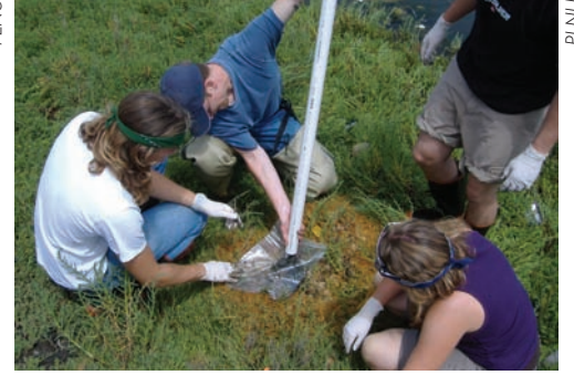
Professor David Cummings of PLNU and undergraduate students extrude a core of channel sediments from Ballona Creek Estuary.
